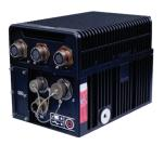
The Rugged Computer RC530 is equipped with the latest iCore processor and superior power management system. It is designed to perform optimally under harsh environments, and comes in a modular form, making it an ideal computer fit even for space-constrained tracked vehicles. It consists of an extensive range of input/output interfaces to support full connectivity for a myriad of peripherals.
