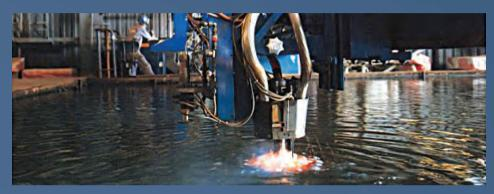
State-of-the-art underwater-plasma cutting machine installed in 1986.
