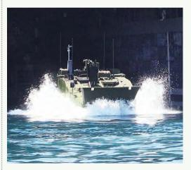
Terrex 2 launching from USS Somerset (LPD-25) in a launch-and-recovery operation trial in 2017.
