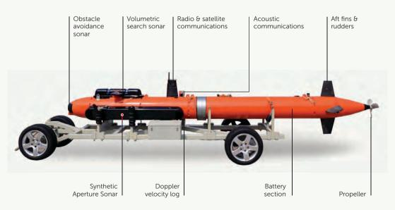
Mercury Autonomous Unmanned Vehicle
