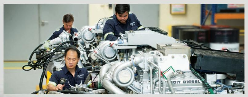
Bionix engine undergoing maintenance at ST Kinetics' component workshop.
