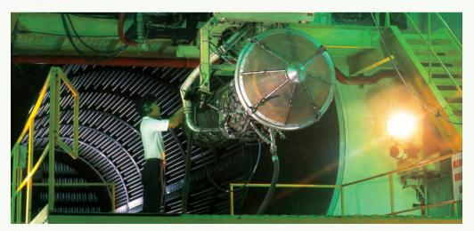
Rigging of a GE J85 engine for testing in the fully computerised test cell of Singapore Aerospace Engines, circa 1990.
