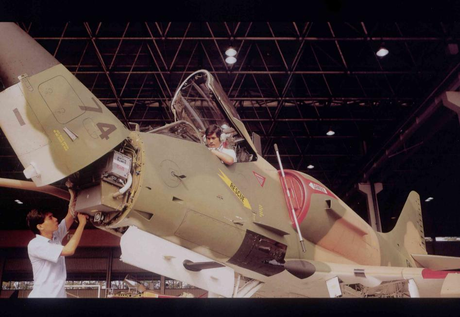
ST Aerospace upgraded the avionics of the A-4 with a state-of-the-art Weapons Delivery and Navigation System.
